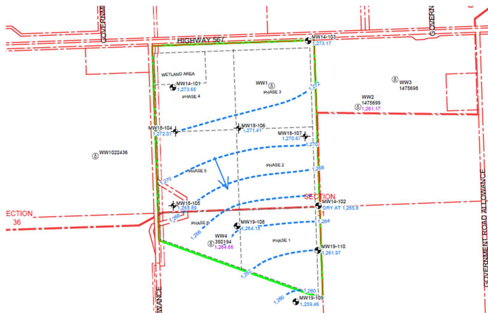
Figure 3. Location of monitoring wells and local water wells (used in the 2020 SLR Hydrogeological Assessment) and mapped water table elevations and contours 6 . (Note: blue arrow indicates direction of flow)
