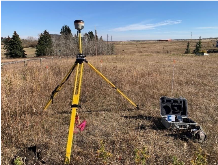
Figure A1: GNSS survey base station set-up. Note that there is a metal pin which the tripod is centered over so that the same base station was used for the multi-day survey.
